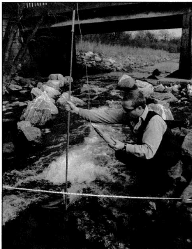
An engineer takes precise measurements of flow velocity after construction at Northwest Branch, allowing him to calculate discharge and determine whether various species can swim upstream.
