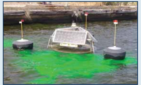
Green tracer dye was used to track the device's range of influence within the water. Engineers monitored dissolved oxygen levels along with water temperature, salinity, density and conductivity in predetermined areas around the mixing and aeration device throughout the summer.
