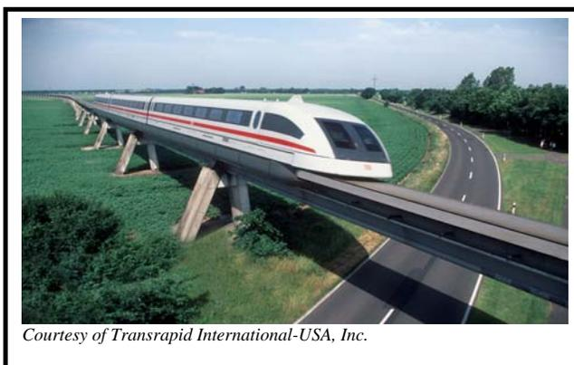
the guideway and permanent magnets housed on the underside of the vehicle. The gap between the top of the guideway and the underside of the vehicle is electronically maintained at about 1 cm (0.4 in) while the vehicle is levitated (Figure 1).
